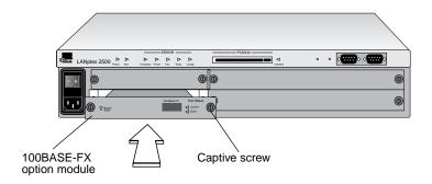
**4** To seat the module, firmly push the module forward to engage the module and backplane connectors. You will feel a slight resistance as the connectors engage.
